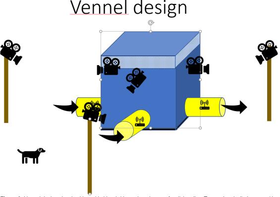
**Figure 3:** Vennel design showing Vennel in blue (with mesh at the top of walls), yellow Tasmanian devil pipe traps (three visible) with trap alerts (with antennae) and wildlife cameras recording animals near traps and approaching Vennel. NOTE: the roof will overhang the walls by about 30cm (not shown above), and the roof and parts of the walls be made from insulation panels to reduce the temperature inside the Vennel.
