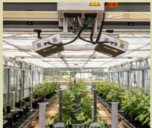
PhenoSpex PlantEye F600: Multispectral LiDAR system captures 3D plant structure & spectral indices
